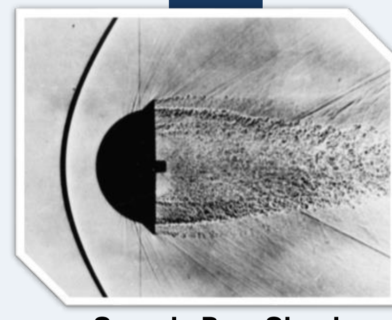
Sample Bow Shock Experienced at Nose (2)
