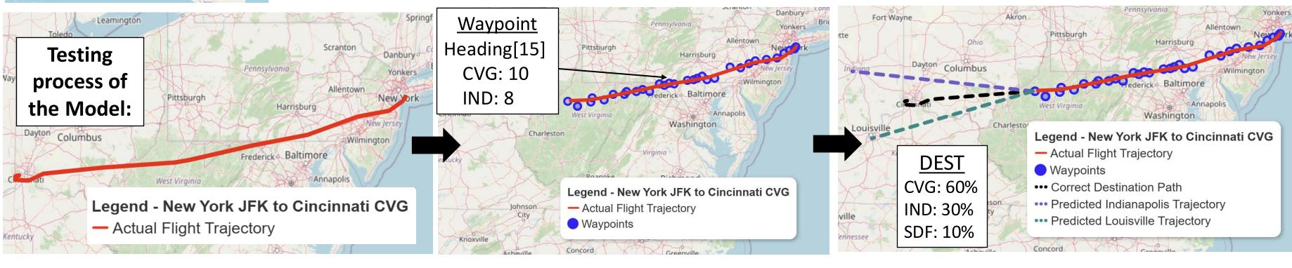
This is a full flight, testing input is any fragment of this, (0 - 60% for this example) Heading is used to search the destination Values used to calculate a sorted list of (Dest, %) map in the bucket of the closest waypoint. for a given number of possible destination.
