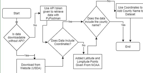
Figure 2: Parameter Retrieval Flowchart
