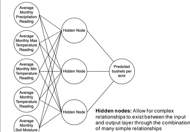
Figure 4: Prediction Model Flowchart
