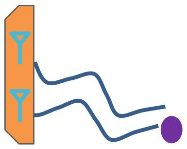
The Bluetooth signal reaches different antennas at different times
