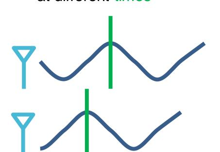
The time difference is used to calculate the angle the beacon is from the locator
