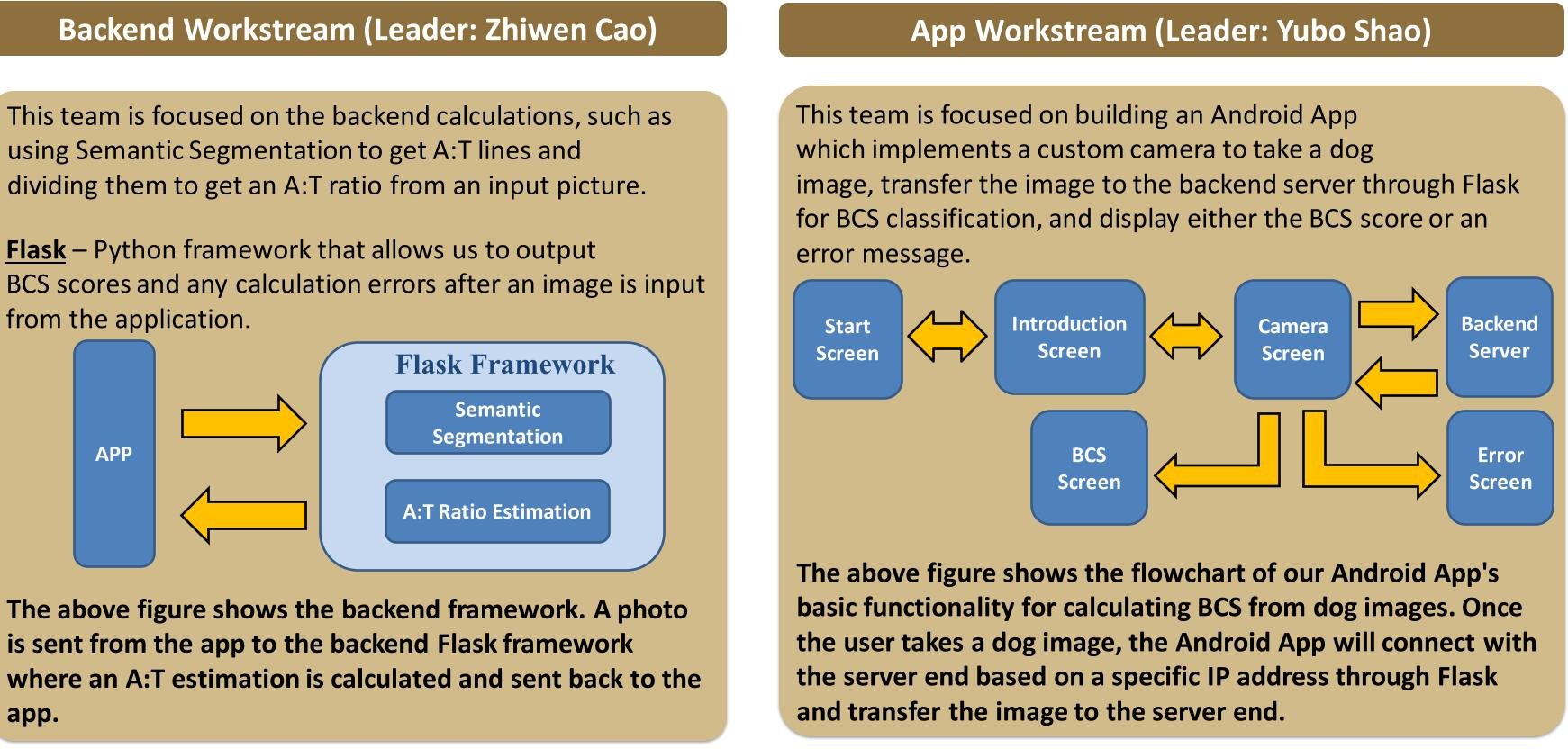
The above figure shows the backend framework. A photo is sent from the app to the backend Flask framework where an A:T estimation is calculated and sent back to the app.
